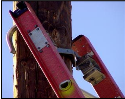
V-Grip supported against pole to prevent turning.
